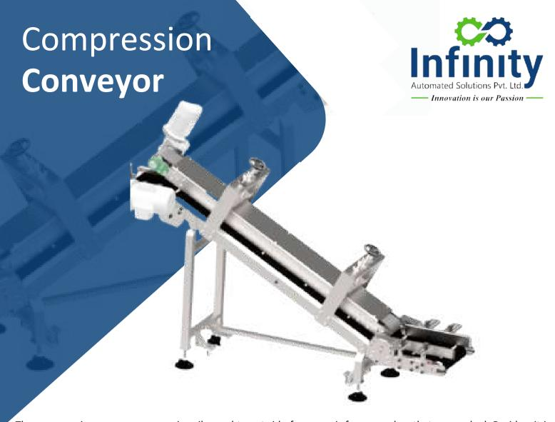
The compression conveyors are primarily used to get rid of excess air from pouches that are packed. Besides, it is also used to flatten the pouch that contains powder or granular products. The sandwich conveyor consists of two conveyors that can be adjusted with a rotating wheel to regulate the pressure and gap between the two conveyors.
